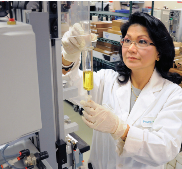
Transformer dissolved gas analysis
