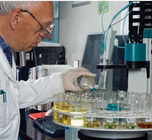
Transformer oil quality testing
