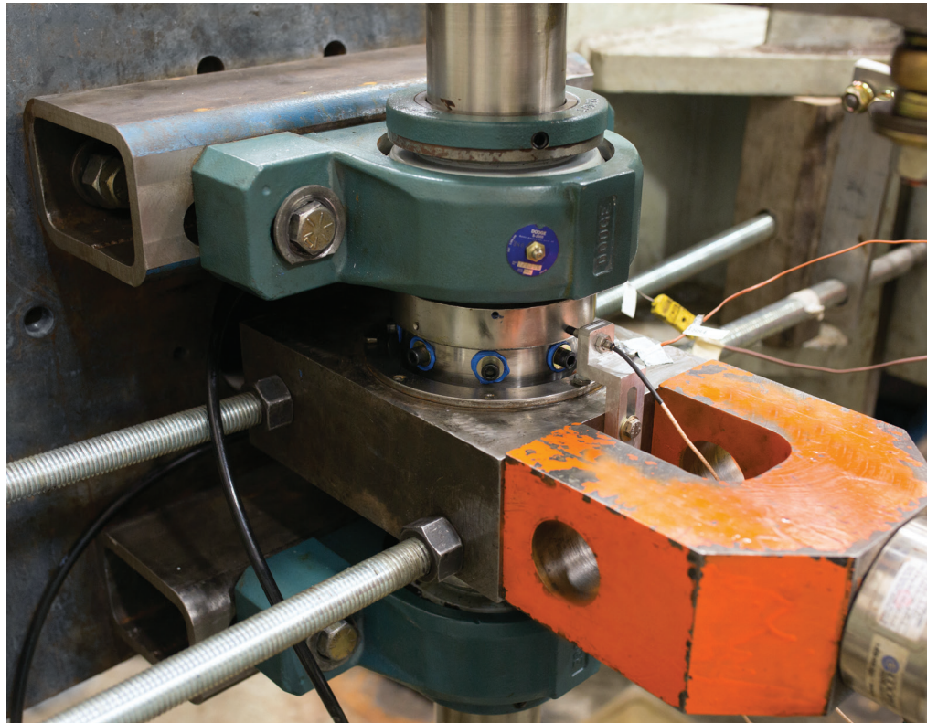
Bearing accelerated wear and friction testing
