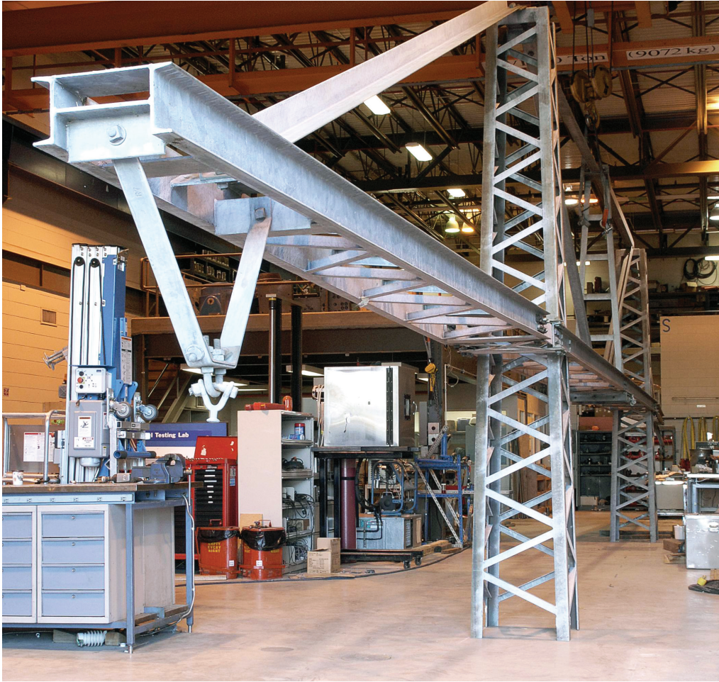
Full-scale load testing of sub-structures
