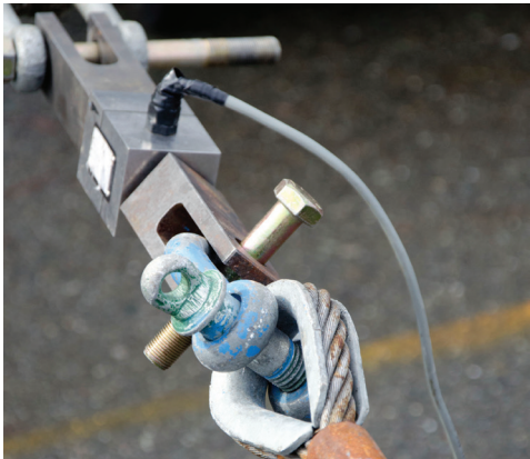
Cable and shackle testing
