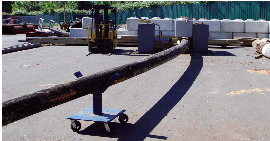
Full-scale wood pole bending test
