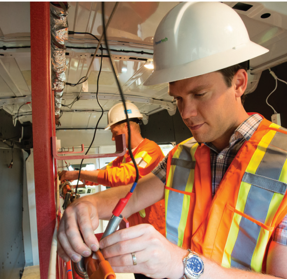
Mobile dielectric testing of insulated tools
