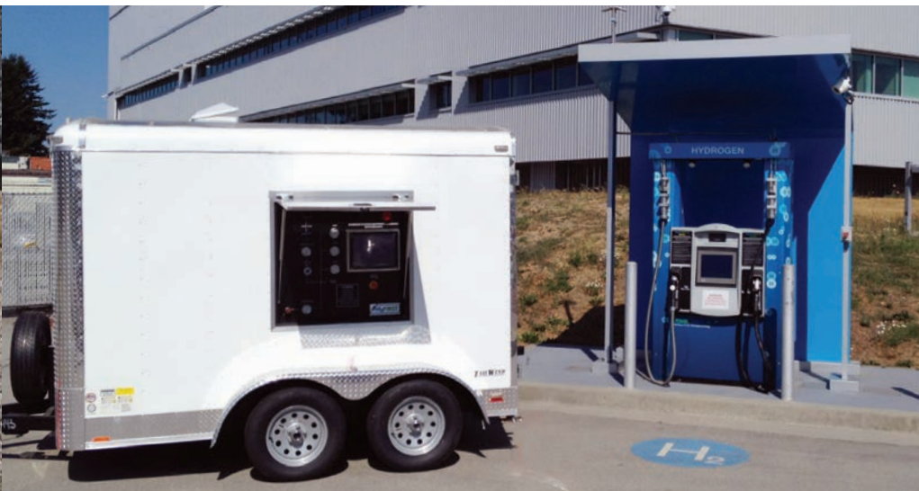
Hydrogen refueling station testing device
