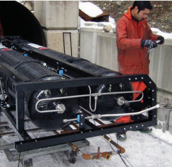
Fire test preparation of bus fuel system
